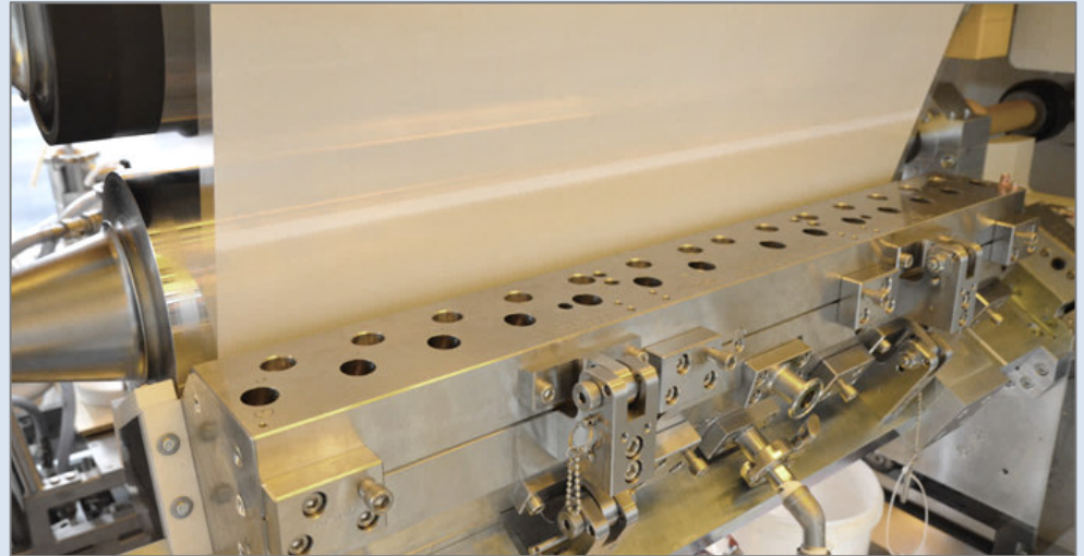
Picture: Dual layer slot die in the technical centre BA2, coating width 1.050 mm
